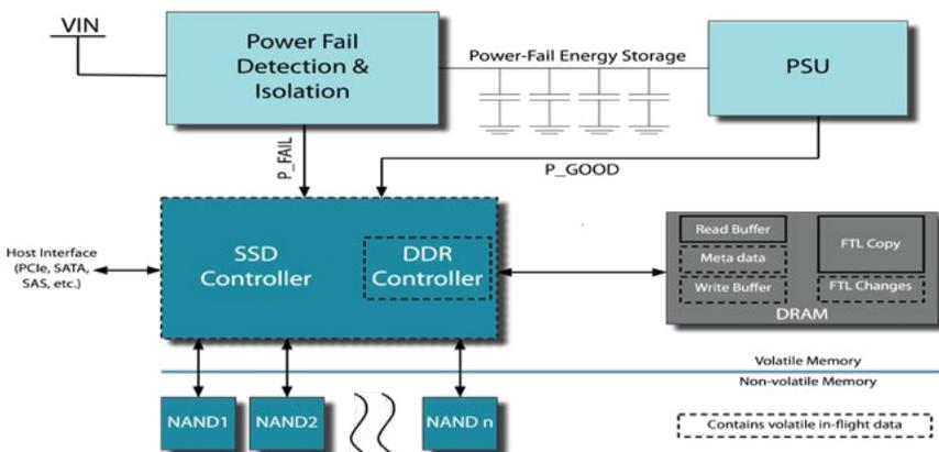
Figure 1: Conventional SSD Architecture with Power Fail Protection
