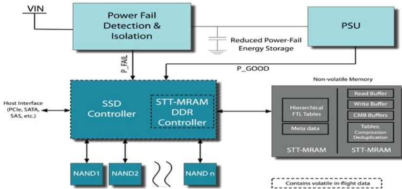
Figure 3: STT-MRAM Replaces DDR in Advanced SSD Architecture
