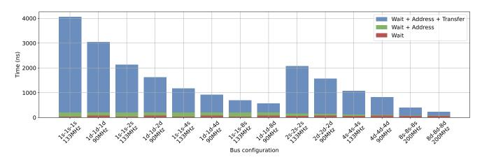
Figure 1: 64-byte long read latency for various bus configurations
