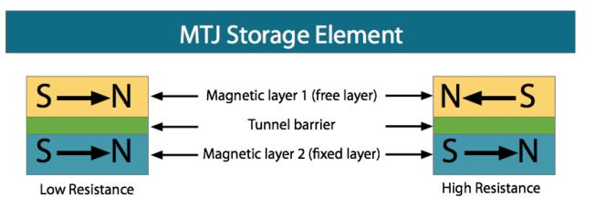
The MTJ device has a low resistance when the magnetic moment of the free layer is parallel to the fixed layer and a high resistance when the free layer moment is oriented anti-parallel to the fixed layer moment. This change in resistance with the magnetic state of the device is an effect known as magnetoresistance, hence the name "magnetoresistive" RAM.
