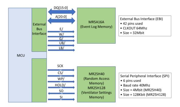
Single or multiple devices can be connected to the SPI bus as shown below. Pins SCK, SO and SI are common among devices. Each device requires CS and HOLD pins to be driven separately.
