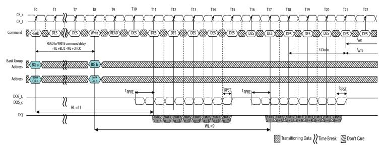
Figure 58 - READ (BL8) to READ (BL8) OTF with 1tCK Preamble in Same or Different Bank Group
