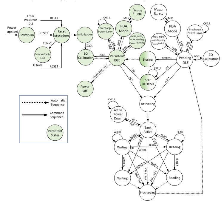
Figure 1 - Simplified State Diagram for ST-DDR4
