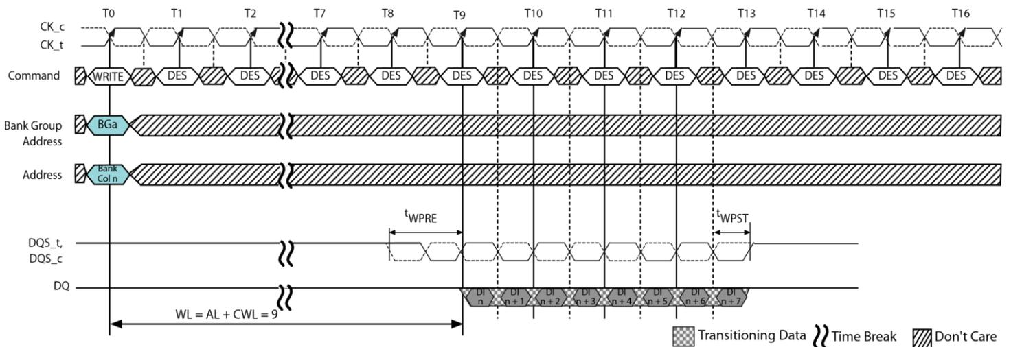
**Figure 71 - WRITE Burst Operation, WL=9 (CWL=9, BL8)**
