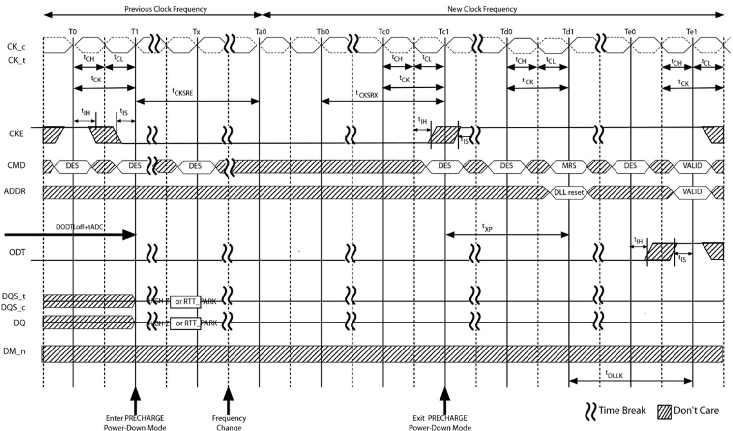
**Figure 18 - Frequency Change During PRECHARGE Power Down**
