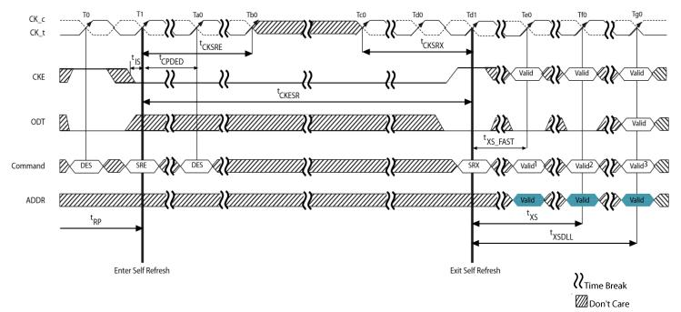
Figure 35 - Self-Refresh Entry/Exit Timing
