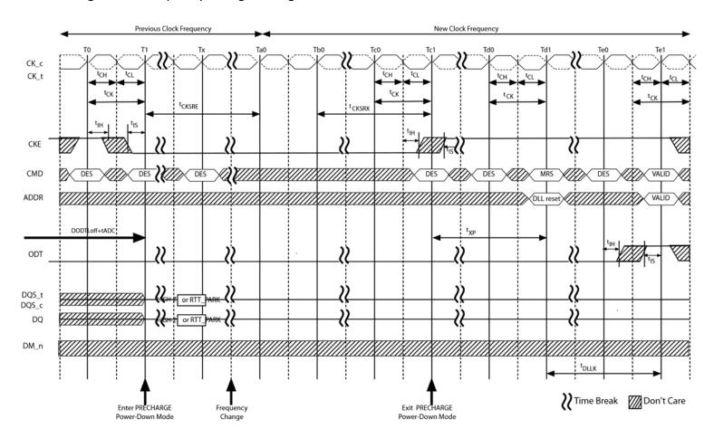
Figure 18 - Frequency Change During PRECHARGE Power Down
