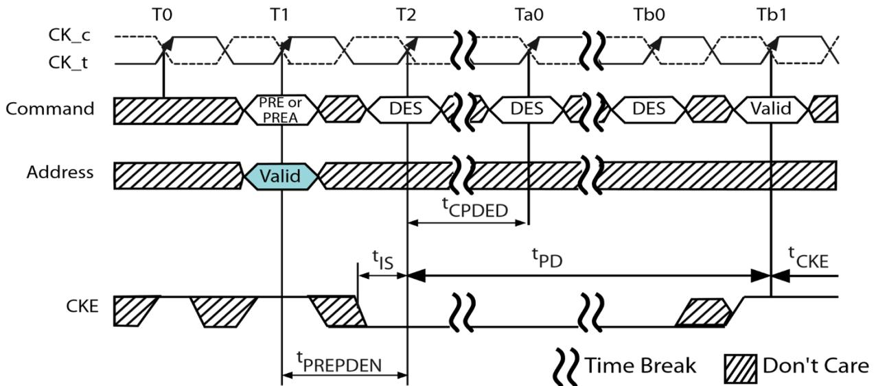
**Figure 43 - PRECHARGE/PRECHARGE ALL Command to Power-Down Entry**
