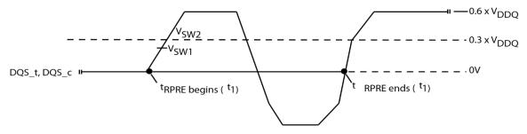
Figure 50 - tRPRE Method for Calculating Transisitions and Endpoints
