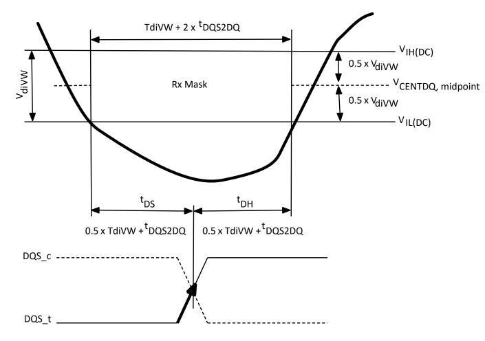
Figure 70 - Example of Data Input Requirements Without Training
