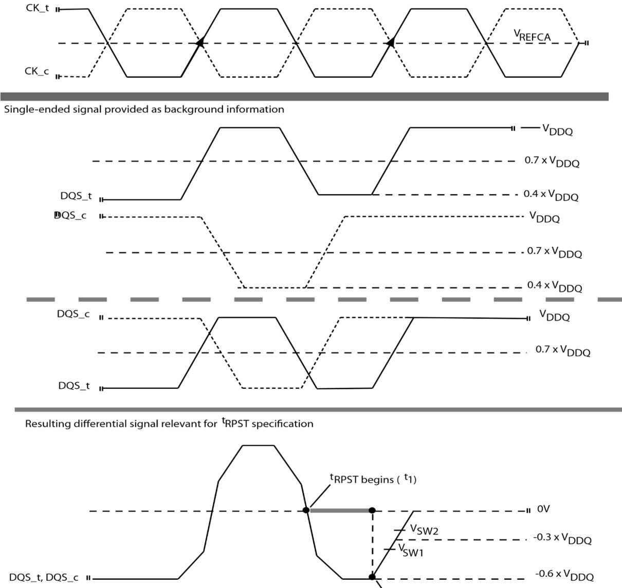
**Figure 51 - t<sub>RPST</sub> Method for Calculating Transitions and Endpoints**
