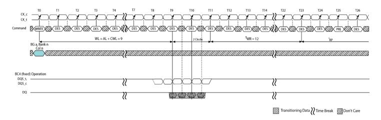
Figure 79 - WRITE (BC4-Fixed) to Auto PRECHARGE with 1tCK Preamble
