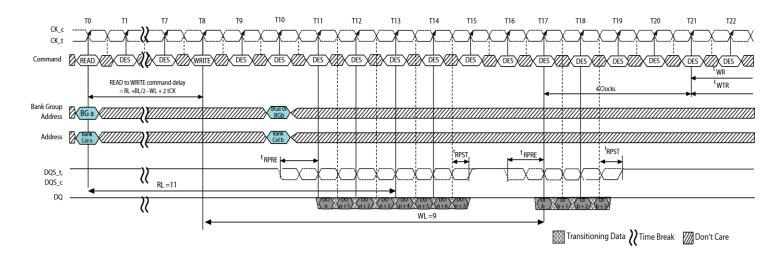
Figure 62 - READ (BL8) to WRITE (BC4) OTF with 1tCK Preamble in Same or Different Bank Group
