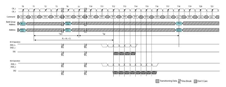
Figure 64 - READ with Auto PRECHARGE and 1tCK Preamble
