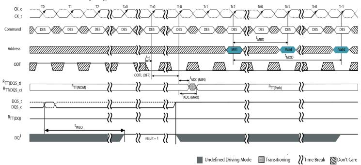
Figure 20 - Write Leveling Exit
