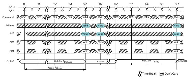
**Figure 80 - ZQ Calibration Timing**
