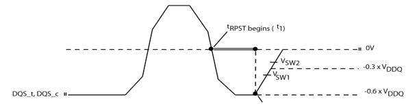
Figure 51 - tRPST Method for Calculating Transisitions and Endpoints
