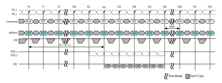
Figure 11 - MPR Read-to-Write Timing
