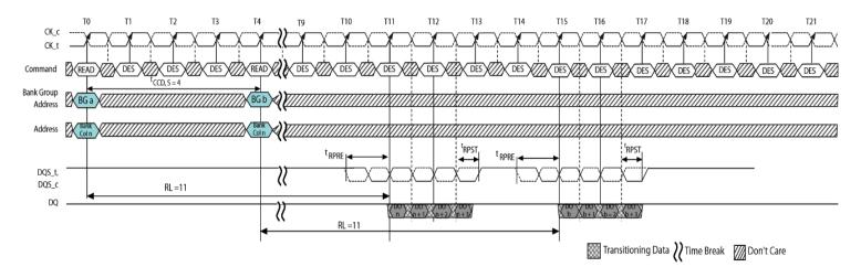
Figure 55 - READ (BC4) to READ (BC4 with 1tCK Preamble in Different Bank Group
