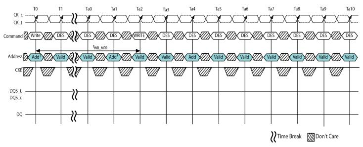
Figure 13 - MPR Back-to-Back Write Timing
