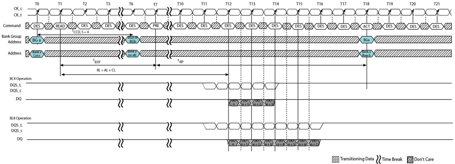
**Figure 63 - READ to PRECHARGE with 1tCK Preamble**
