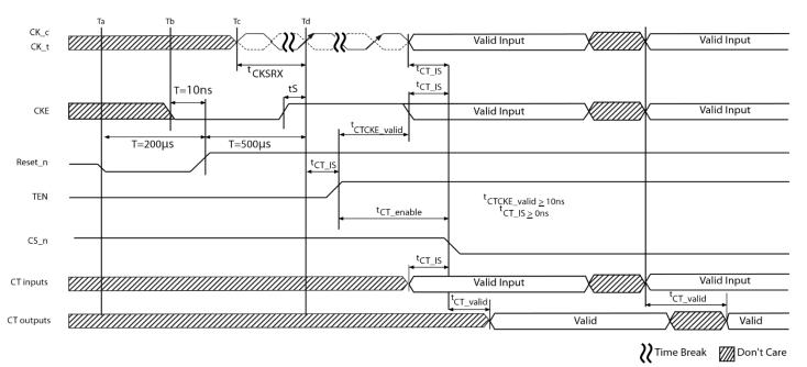
**Figure 32 - Connectivity Test Mode Entry**
