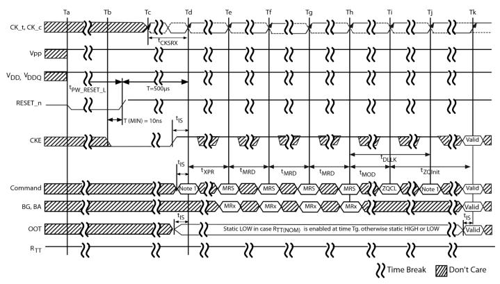
Figure 5 - Reset and Initialization Sequence at Power-On Ramping
