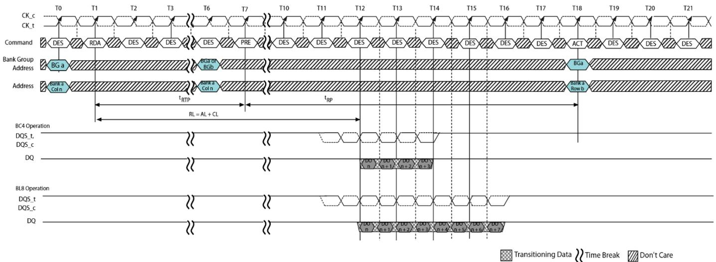
**Figure 64 - READ with Auto PRECHARGE and 1tCK Preamble**
