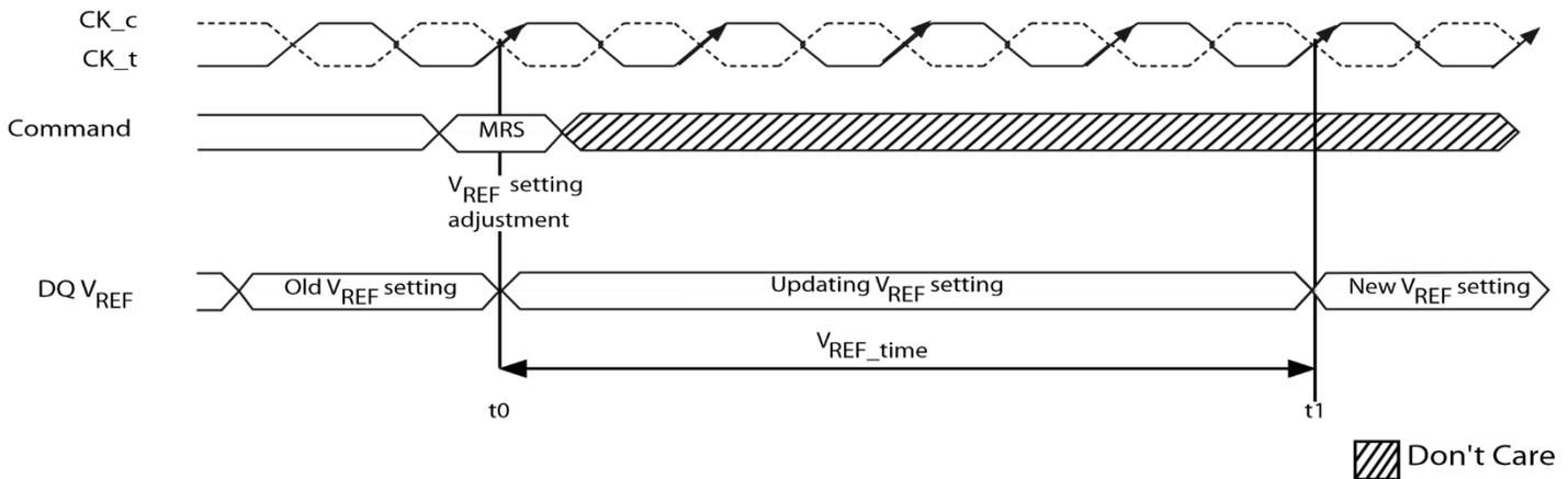
**Figure 25 - VREFDQ Timing Diagram for VREF,time Parameter**
