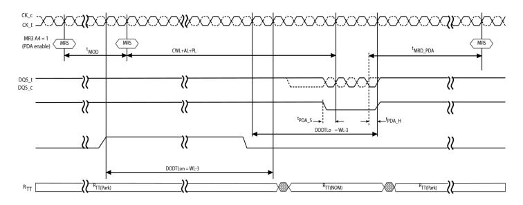
Figure 21 - PDA Operation Enabled, BL8
