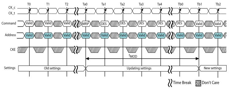
Figure 8 - t<sub>MOD</sub> Timing
