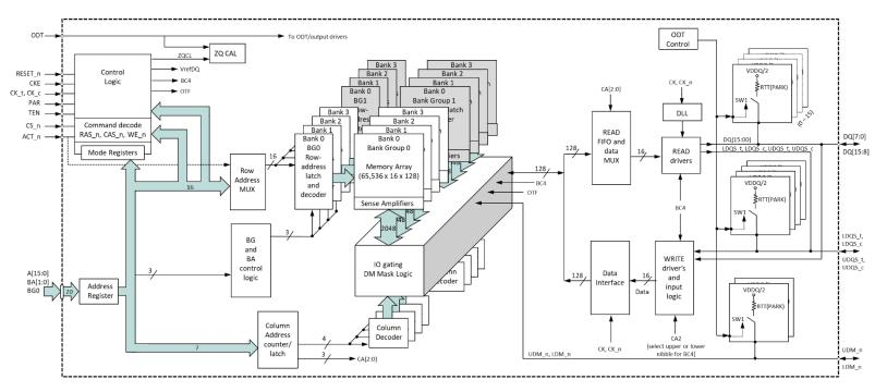
Figure 3 - Functional Block Diagram for 1Gb x16 ST-DDR4
