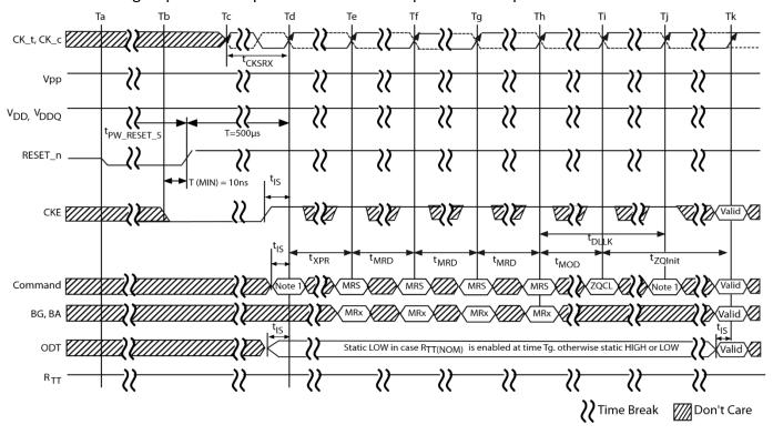
**Figure 6 - Reset with Stable Power**
