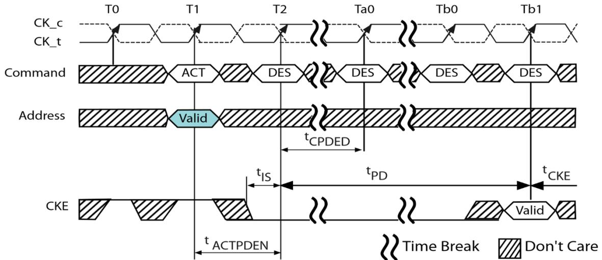
**Figure 42 - ACTIVE Command to Power-Down Entry**
