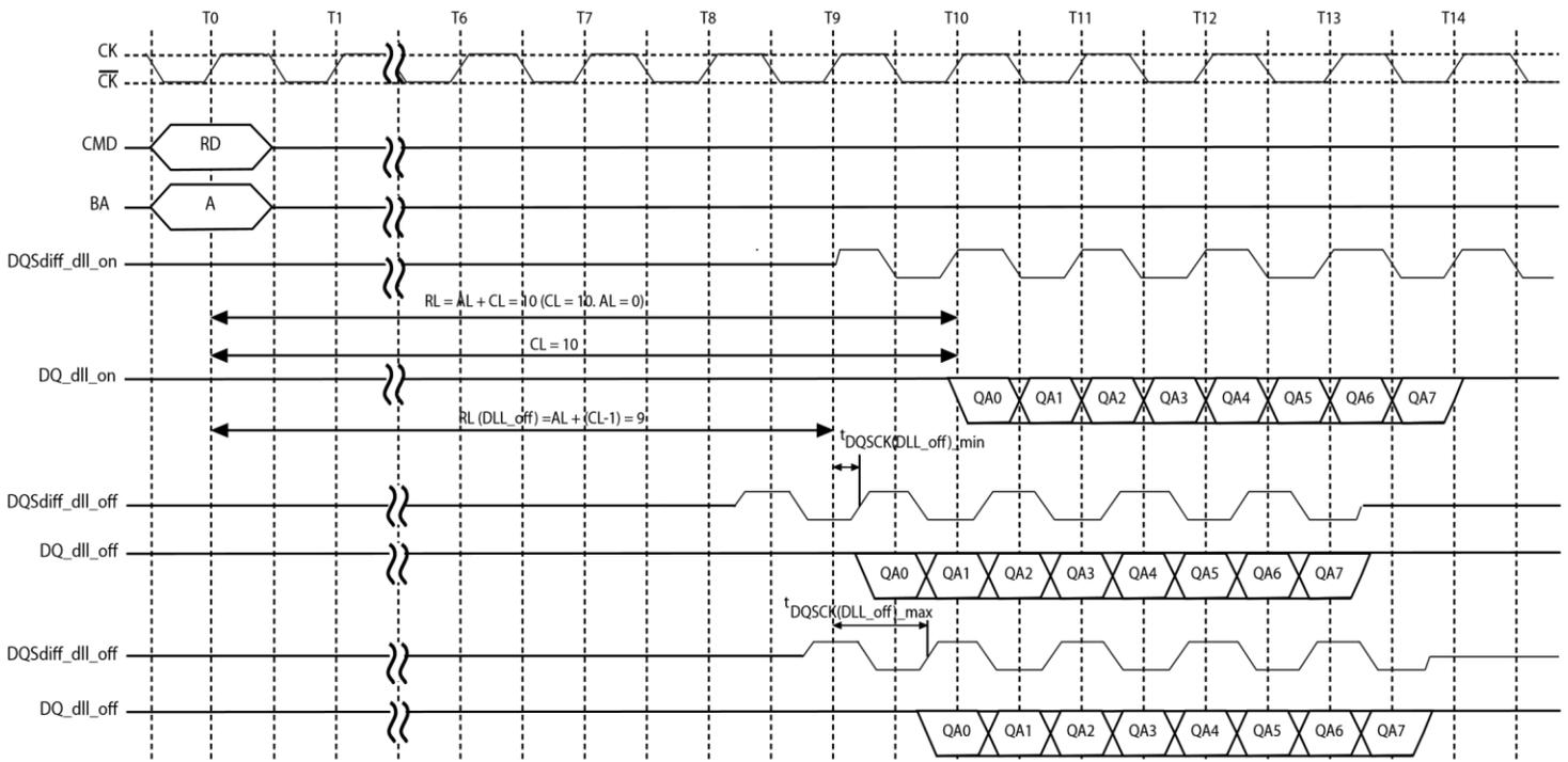
**Figure 17 - Read Operation in DLL Off Mode**
