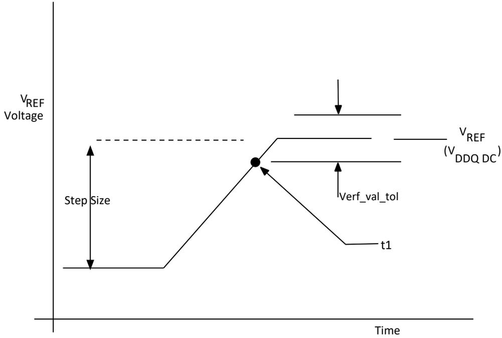
**Figure 27 - VREF Single Step Size Increment Case**
