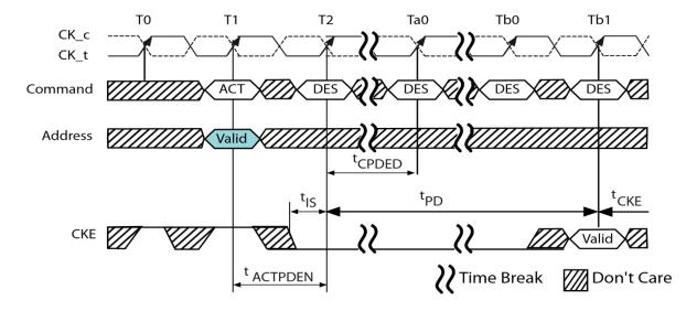
Figure 42 - ACTIVE Command to Power-Down Entry
