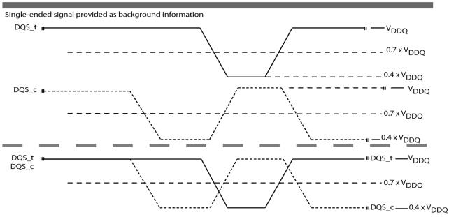
Resulting differential signal relevant for <sup>t</sup>RPRE specification
