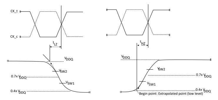
Figure 49 - tLZ, and tHZ(DQS) Method for Calculating
