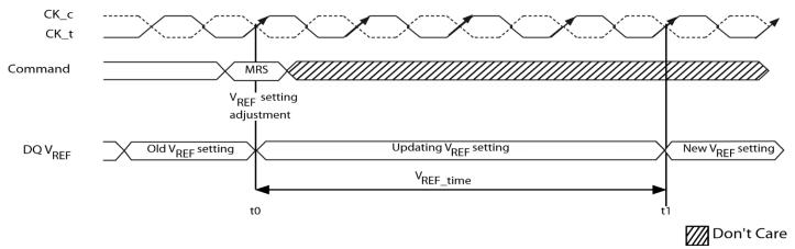
Figure 25 - VREFDQ Timing Diagram for VREF,time Parameter
