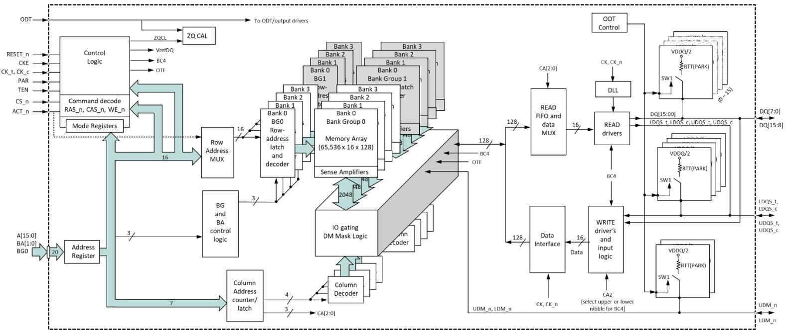
Figure 3 - Functional Block Diagram for 1Gb x16 ST-DDR4
