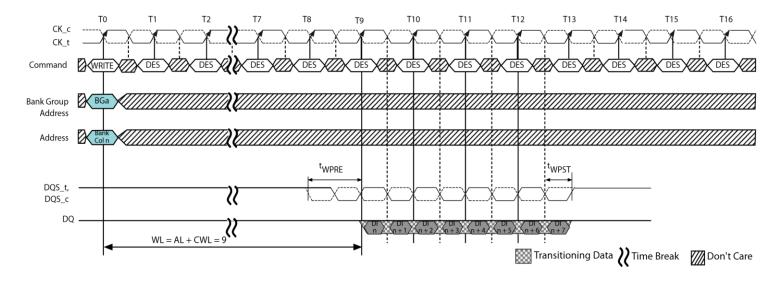
Figure 71 - WRITE Burst Operation, WL=9 (CWL=9, BL8)
