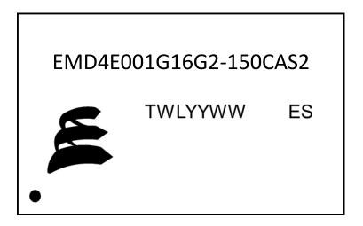
Figure 82 - Part markings showing example OPN
