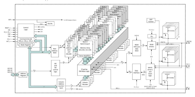
Figure 2 - Functional Block Diagram for 1Gb x8 ST-DDR4
