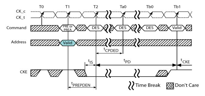
Figure 43 - PRECHARGE/PRECHARGE ALL Command to Power-Down Entry
