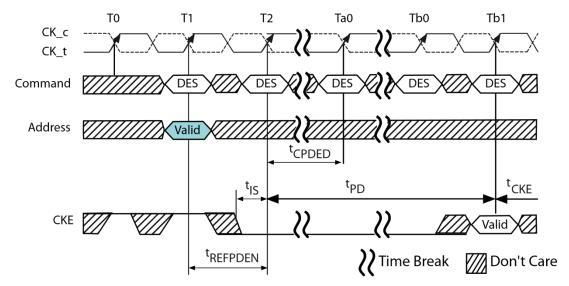
Figure 41 - REFRESH Command to Power-Down Entry
