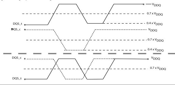
Resulting differential signal relevant for <sup>t</sup>RPST specification
