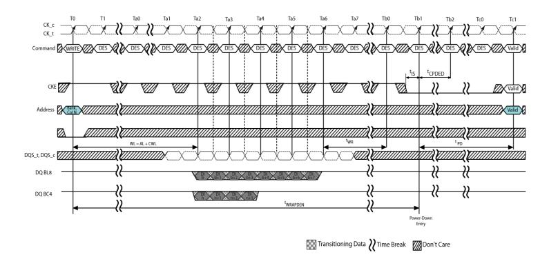
Figure 39 - Power-Down Entry After Write
