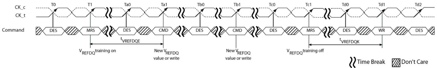
**Figure 26 - Training Mode Entry and Exit Timing Diagram**
