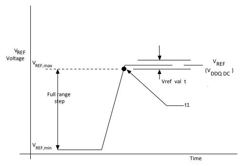
Figure 29 - VREF Full Step: VREF,min to VREF,max
