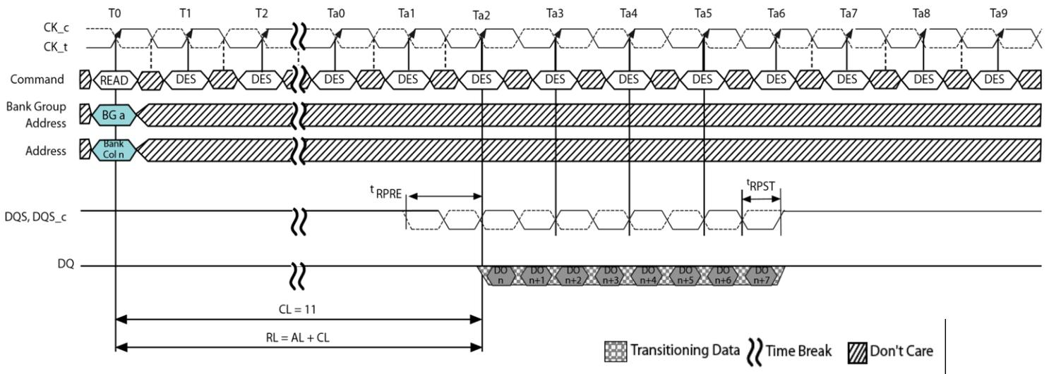
**Figure 52 - READ Burst Operation, RL = 10 (CL = 10, BL8)**
