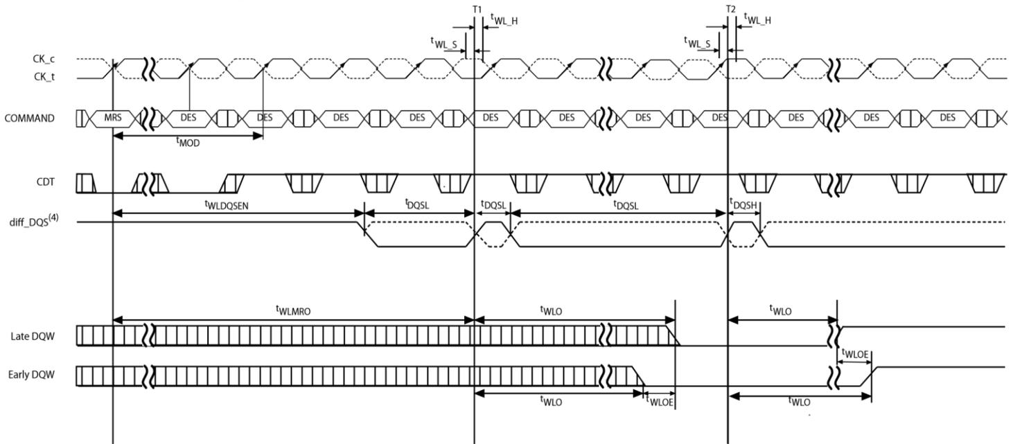
**Figure 19 - Timing details of the Write Leveling Sequence**
