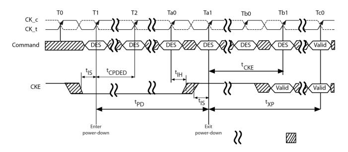
Figure 40 - Precharge Power-Down Entry and Exit
