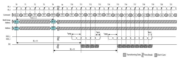
Figure 57 - READ (BC4) to READ (BL8) OTF with 1tCK Preamble in Different Bank Group
