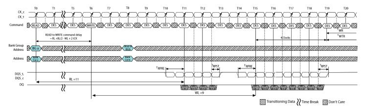
Figure 61 - READ (BC4) to WRITE (BL8) OTF with 1tCK Preamble in Same or Different Bank Group
