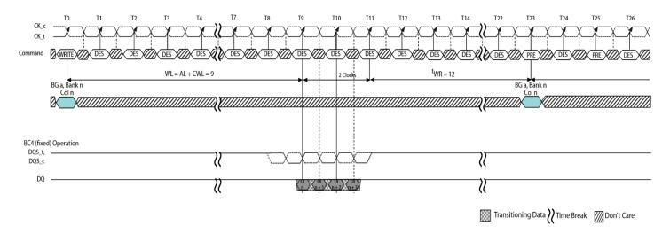
Figure 77 - WRITE (BC4-Fixed) to PRECHARGE with 1tCK Preamble
