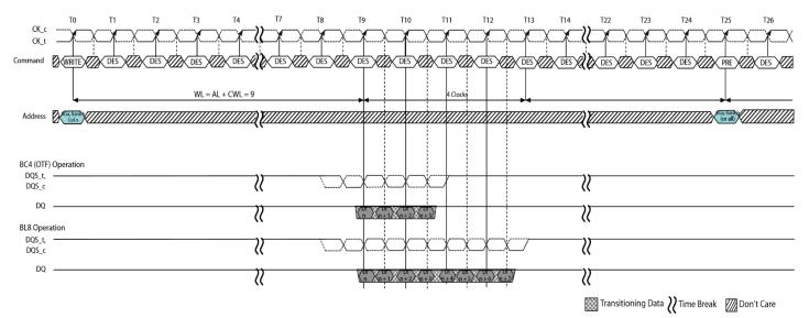
Figure 76 - WRITE (BL8/BC4-OTF) to PRECHARGE with 1tCK Preamble
