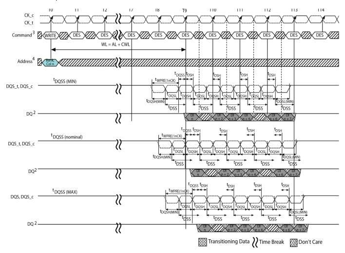
**Figure 65 - WRITE Timing Definition**
