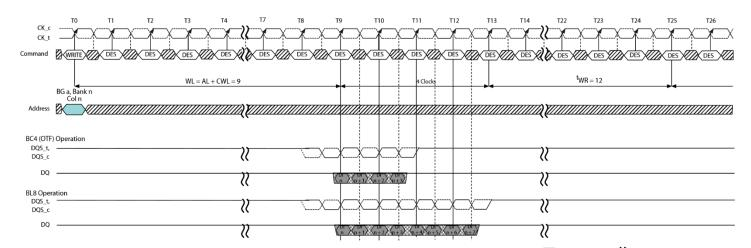
Figure 78 - WRITE (BL8/BC4-OTF) to Auto PRECHARGE with 1tCK Preamble
