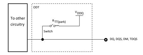
**Figure 81 - Functional Representation of ODT**
