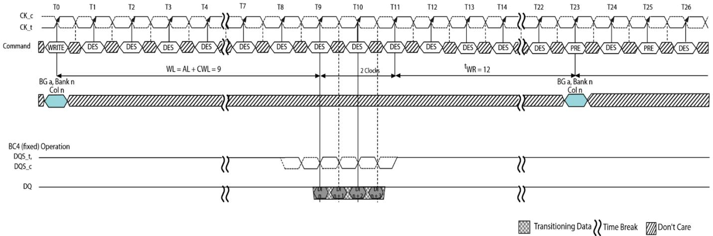
**Figure 77 - WRITE (BC4-Fixed) to PRECHARGE with 1tCK Preamble**
