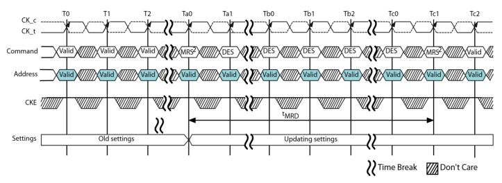
Figure 7 - t<sub>MRD</sub> Timing
