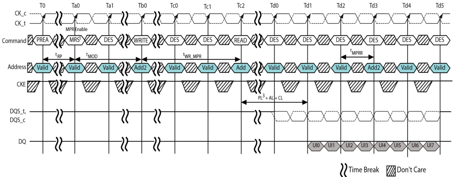
**Figure 12 - MPR Write and Write-to-Read Timing**
