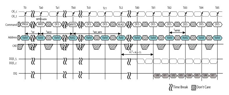
Figure 12 - MPR Write and Write-to-Read Timing
