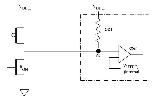
Figure 31 - VREFDQ Equivalent Circuit
