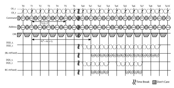
Figure 10 - MPR Back-to-Back Read Timing
