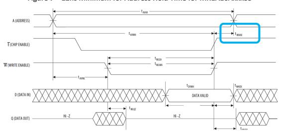
Figure 7 – 12ns Minimum for Address Hold Time for MR1A16Axxx35
