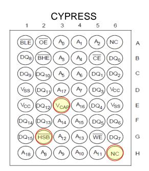
Figure 2 - Pinout comparison between MRAM and nvSRAM, 48 FBGA package
