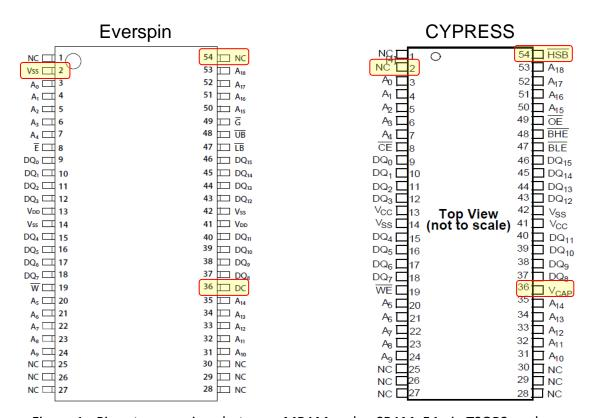
Figure 1 - Pinout comparison between MRAM and nvSRAM, 54 pin TSOP2 package
