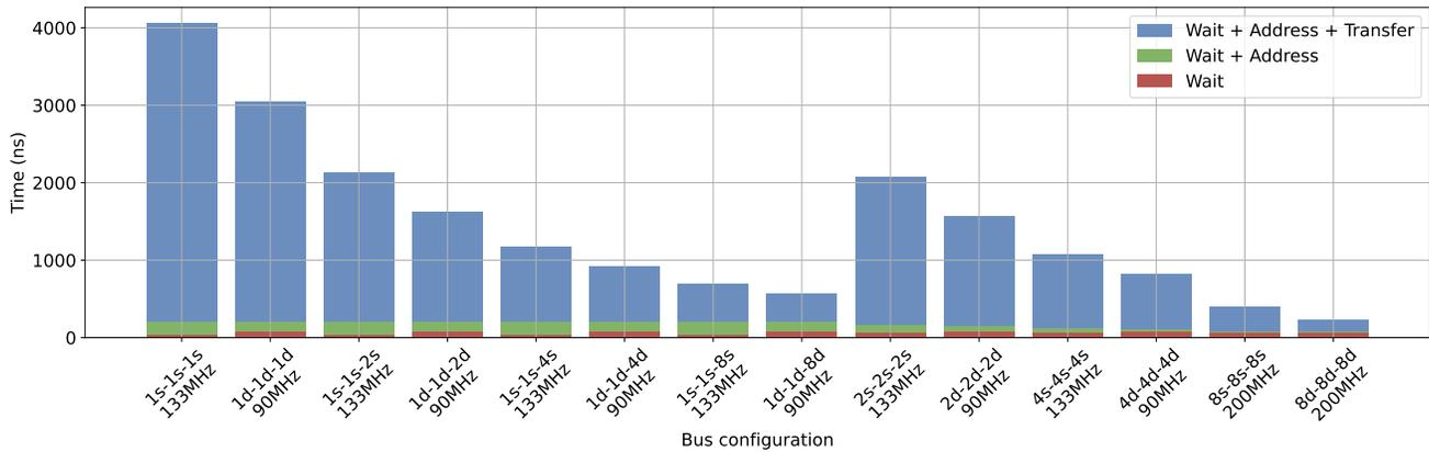
Figure 1: 64-byte long read latency for various bus configurations
